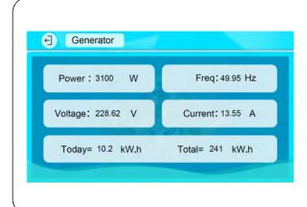
Click the generator icon at the bottom of the main page to view the current generator parameters (the generator is not enabled)
