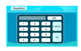
On the basic settings page P1, select "Lock out all changes" and click . In the pop-up window, enter the user password to complete the setting. All setting parameters cannot be set, but can only be viewed. To unlock, select the function again and enter the user password to unlock.
