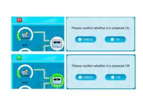
Check "Manual Swith" on page P1 of the basic settings and click the leave button (close to uncheck the settings).
